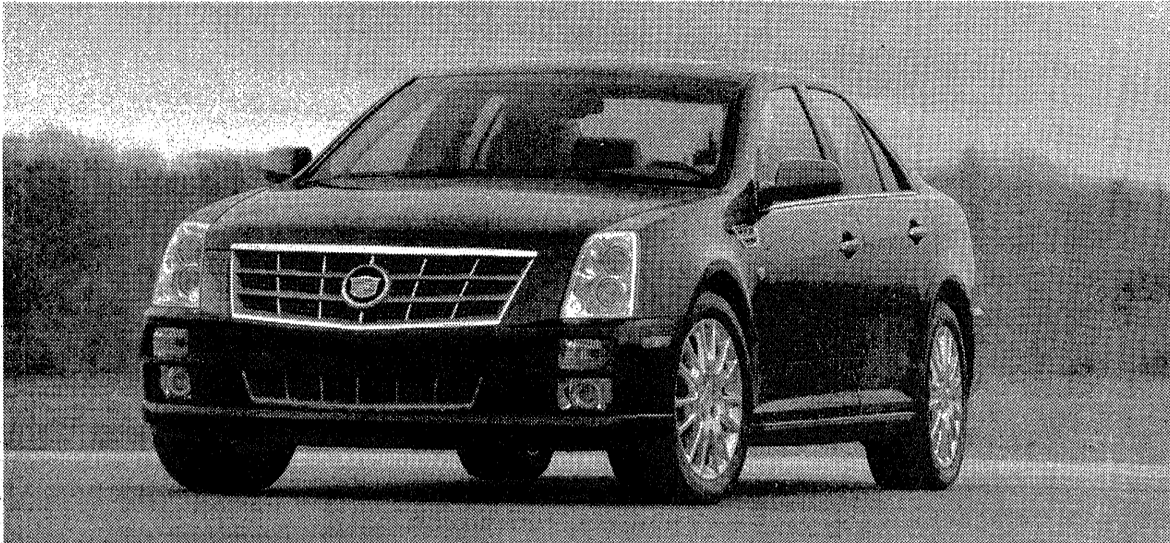
The Cadillac STS is debuting General Motors' new 3.6-liter direct injection V6 engine this year. It pushes the STS's horsepower up from 255 to 298.
