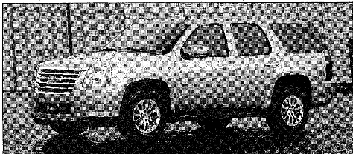
The 2008 Yukon Hybrid, along with the 2008 Chevrolet Tahoe Hybrid, are the world's first SUVs with a dual-motor, two-mode hybrid system. This upped the fuel economy rating by 25 percent over the traditional Yukon.
