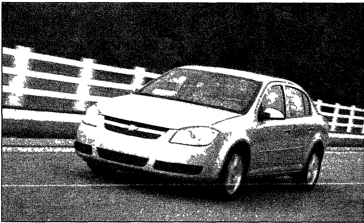
2005 Chevrolet Cobalt. Vehicle class: Subcompact coupe or sedan. Power: 2.2-liter dual overhead cam inline four cylinder. Fuel economy: 24 mpg city/ 32 mpg highway. Where built: Lordstown, Ohio. Price as tested: $19,495.
