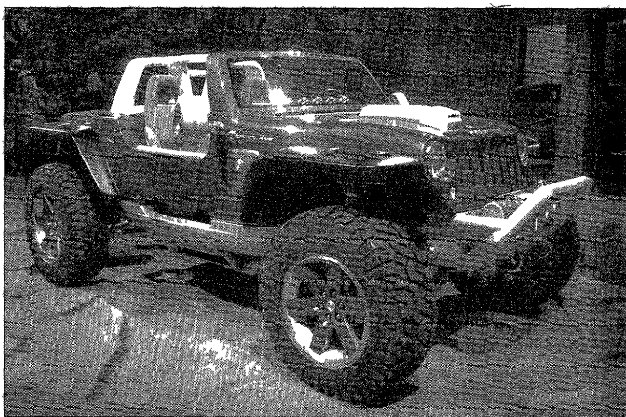
The Jeep Hurricane is an off-road concept vehicle taken to the extreme. It has two Hemi engines and four-wheel steering that enables it to turn within its own length.
