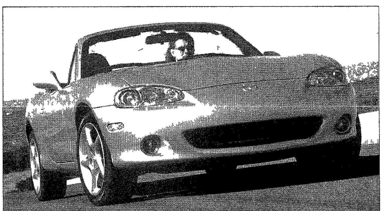
2003 Mazda Miata. Vehicle type: Compact sports car. Power: 1.8 liter dual overhead cam four cylinder engine. Mileage: 23 mpg city / 28 mpg highway. Horsepower: 142 horsepower. Where built: Japan.
