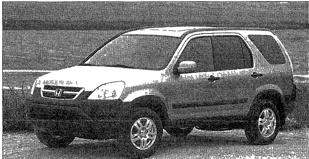
2003 Honda CR-V. Vehicle type: Special purpose vehicle. Power: 2.4-liter DOHC 16-valve 4-cylinder engine. Mileage: 22 mpg city/26 mpg highway. Where built: Sayama, Saitama, Japan. Price as tested: $22,860.
