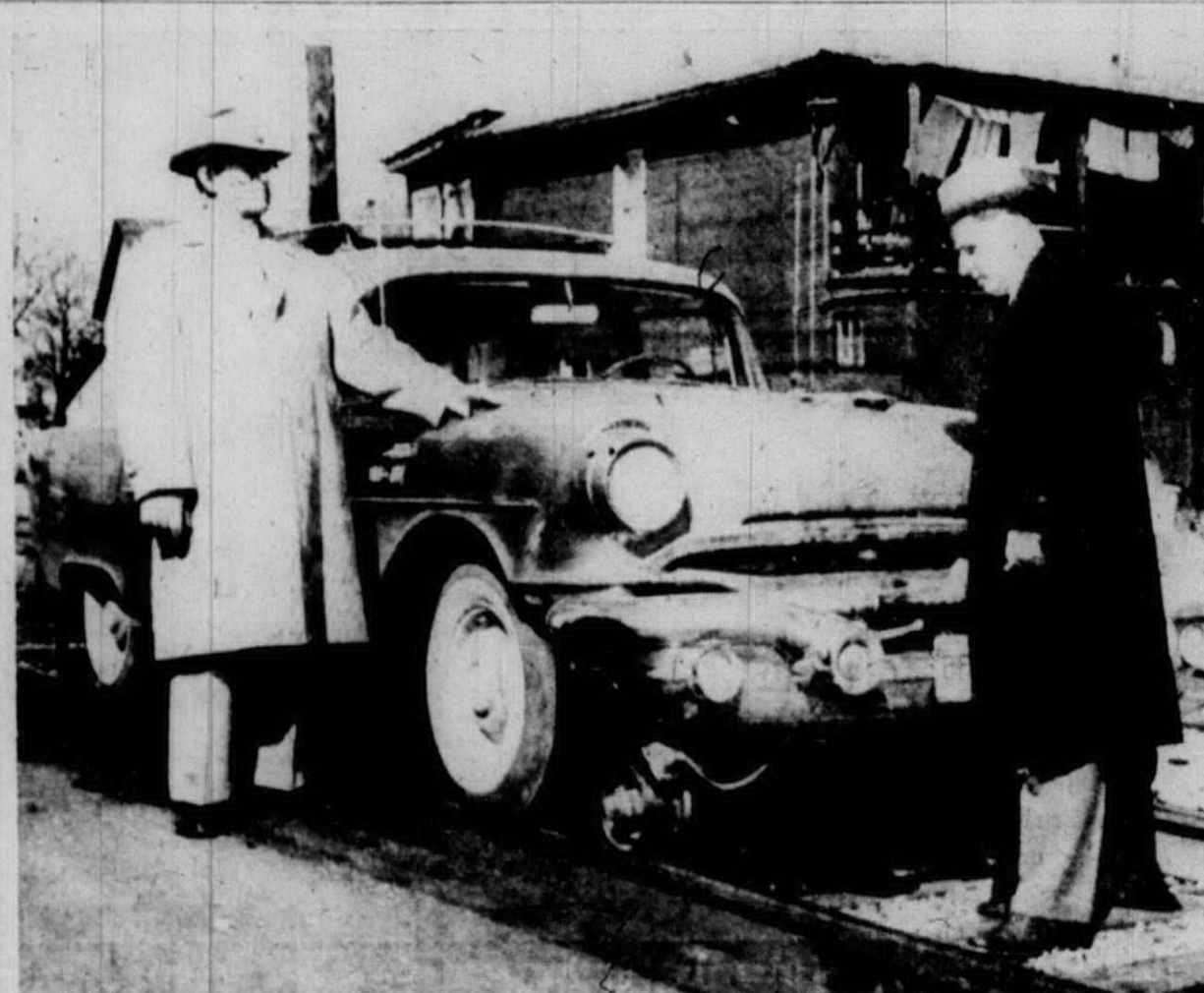
MOST PEOPLE take a second look when they see a Pontiac station wagon coming down the C & O Railroad tracks. Called a Hy-Rail car, the vehicle is used for inspection purposes by railroad officers between Detroit and Grand Rapids. The flanged railroad wheels are retractable, making it possible for use on the highway. This is the only one of its kind on the C & O. Pictured with the car in Plymouth last week are Robert Fenton, freight and passenger agent, left; and J. N. Ikner, trainmaster for the Detroit Terminal.
