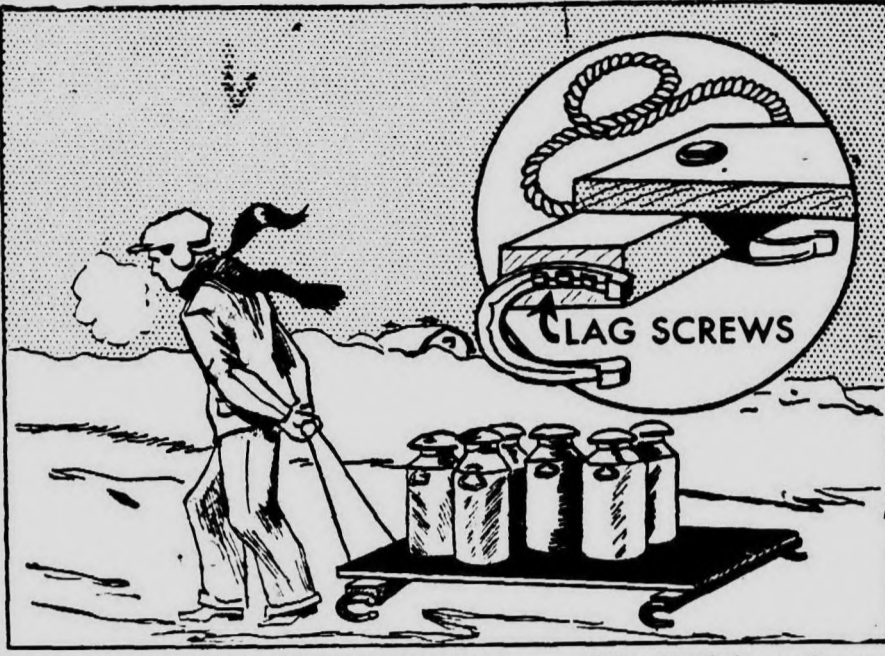
HORSESHOES AS SLED RUNNERS . . . Discarded horseshoes, attached to a sled by means of small lag screws, make good runners for a small sled that is used about farm buildings for simple chores. Holes in shoes are enlarged to receive the screws.
