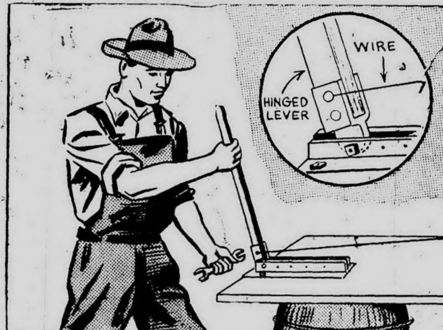
Wire removed from bales of hay, straw, etc., has many uses. Straighten with simple hand stretcher shown, which consists of long plank having lever mounted on one end, hook on the other. Lever bolted between angle iron pieces.
