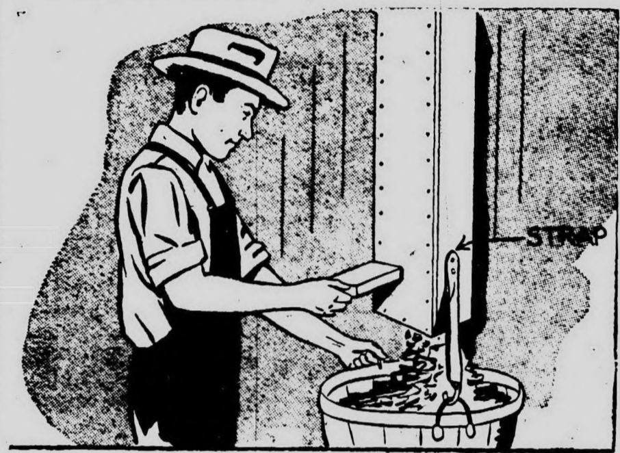
A strap with hook on end makes it possible to hold a large basket under a grain spout with one hand so shutoff slide may be operated with the other.
