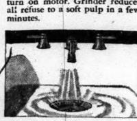
Water from the tap washes away the finely ground material.
