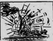
THE FIRST LOCOMOTIVE EXPLOSION IN THE UNITED STATES OCCURRED IN 1839 ON THE CHARLESTON AND HANBROG LINE IN SOUTH CAROLINA. WHEN THE LOCOMOTIVE "BEST FRIEND" BLEW UP AFTER THE FIRE-MAN TIED DOWN THE SAFETY VALVE BECAUSE HE DIDN'T LIKE THE HISSING SOUND.
