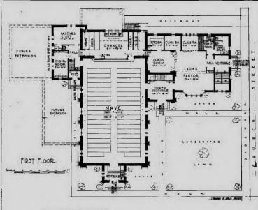
DANQUET HALL. Details of the floor plan for the new Presbyterian church are shown above in the drawings by Thomas W. Moss architect. The exterior of the building will be of seventeenth century Gothic architecture, the main auditorium being 40 by 80 feet.
