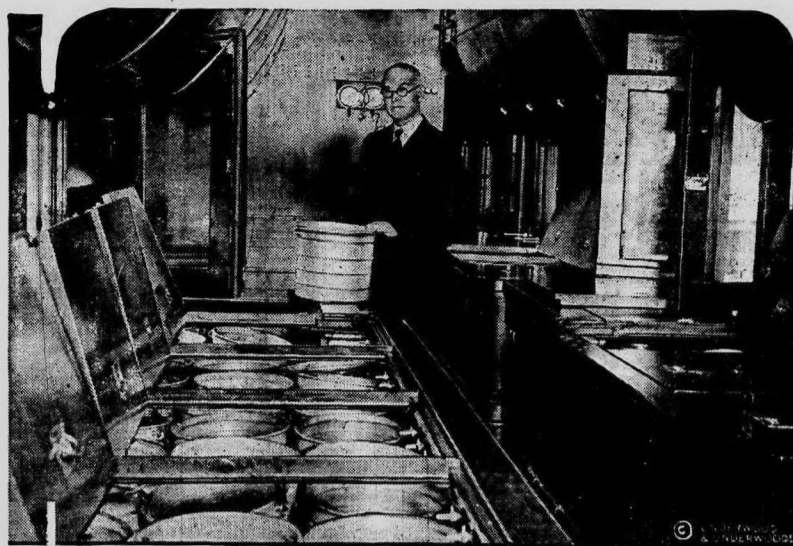
A new de luxe all-steel car for the transportation and distribution of young fish has just been put in service by the bureau of fisheries at Washington. The car resembles a conventional pullman and is fitted with tanks which will contain half a million young fish, in addition to living quarters for the crew of caretakers who accompany the fishy passengers. The photograph shows E. C. Fearnow, superintendent of distribution of the bureau, examining some of the tanks.
