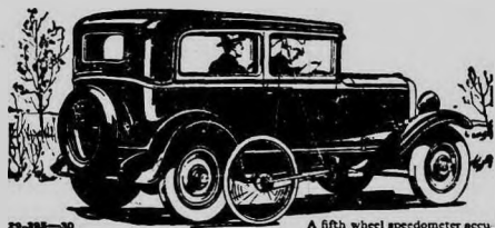
A fifth wheel speedometer accurately measures speed and mileage on all Chevrolet test runs at the Proving Grounds.
