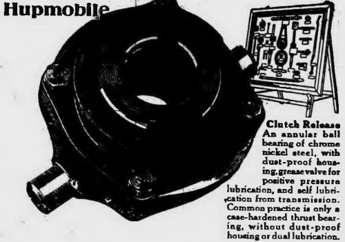
Clutch Release An annular ball bearing of chrome nickel steel, with dust-proof housing, grease valve for positive pressure lubrication, and self lubrication from transmission. Common practice is only a case-hardened thrust bearing, without dust-proof housing or dual lubrication.
