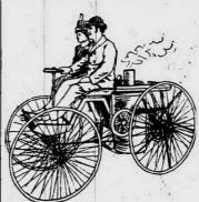
Steam can be made in five minutes. steering wheel is provided in front of the seat. The exhaust steam is passed through a feed water heater, and is then delivered to the naptha flame. where its presence destroys noise. No skill is needed in the management of the wagon, and it can make ten miles an hour and climb hills with two passengers -- Scientific American.
