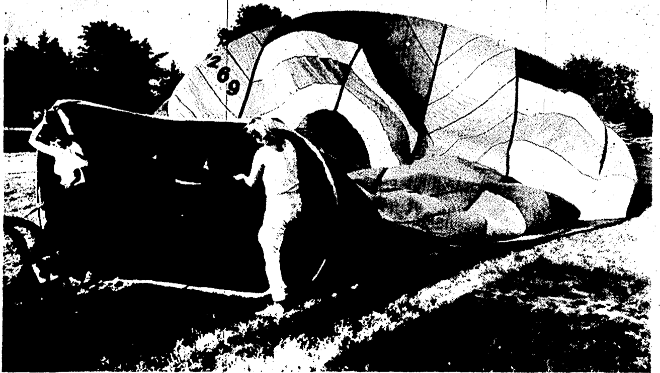
A small, motorized fan is positioned to inflate the balloon. A jet burner then provides the hot air for lift-off.
